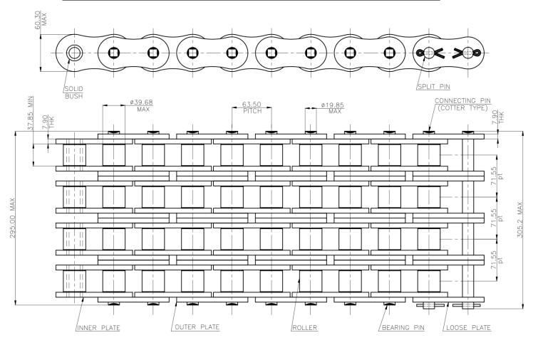
MINIMUM BREAKING LOAD = 185400 kgs(1818.77 KN)
